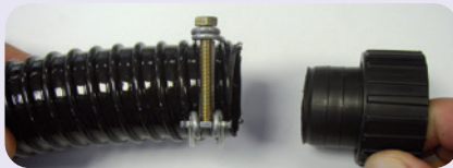
Put clip on hose and then hose on tail
