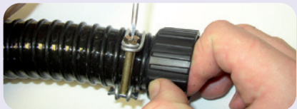
Tighten up clip to make it watertight
